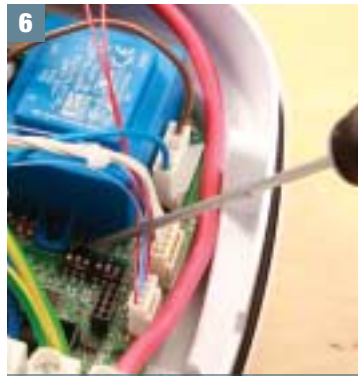
PLEASE NOTE! The shower is factory set with the 'DIP Switch' set for Eco performance – consult user should any other options be preferred. (See Page 6 for details)
