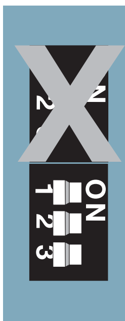
PLEASE NOTE! The Selectronic Premier is factory set with 'DIP Switch' set for Eco showering.
